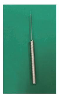
When the temperature of the nozzle is raised and the UI as shown below is displayed, insert the nozzle spring pin at the nozzle inlet side and turn it to the left and right to drill it.
