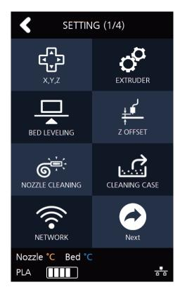
3 Entering Cleaning Case, the nozzle will automatically position itself to the left side to be visible and accessible. Like shown in the image, empty the CASE, press **[OK]** when done and user will be returned to the settings screen.
